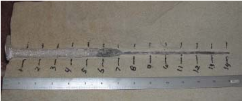
(b) Figure b shows the effective length of the perforation, when a stressed Castlegate sandstone core was shot at balanced conditions and subsequently flow tested. The effective length of the perforation which would flow was only 7 in. (18 cm), although the perforation penetrated 14 in. (35 cm).
