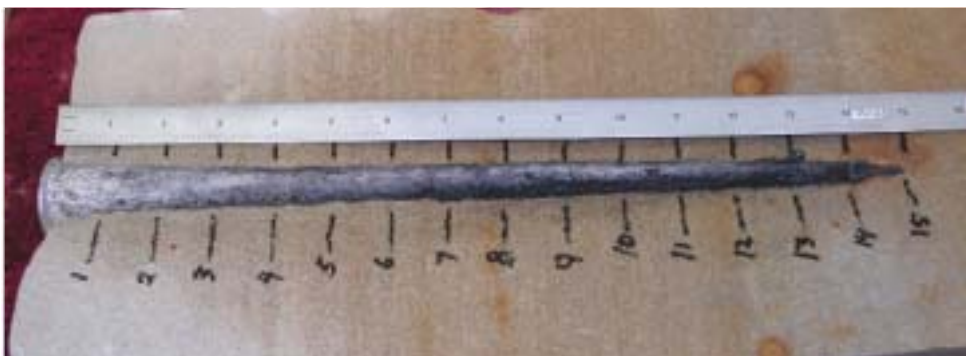
(c) Figure c shows the effective length of the perforation, when a stressed Castlegate sandstone core was shot with 3500 psi (22 MPa) underbalance pressure and subsequently flow tested. The effective perforation would flow almost its entire length of 15 in. (38 cm). It is important to note that 3500 psi (22 MPa) underbalance, generally considered an extremely high level, in this high permeability sandstone with liquid filled pore space, and cannot always be achieved for operational reasons.
