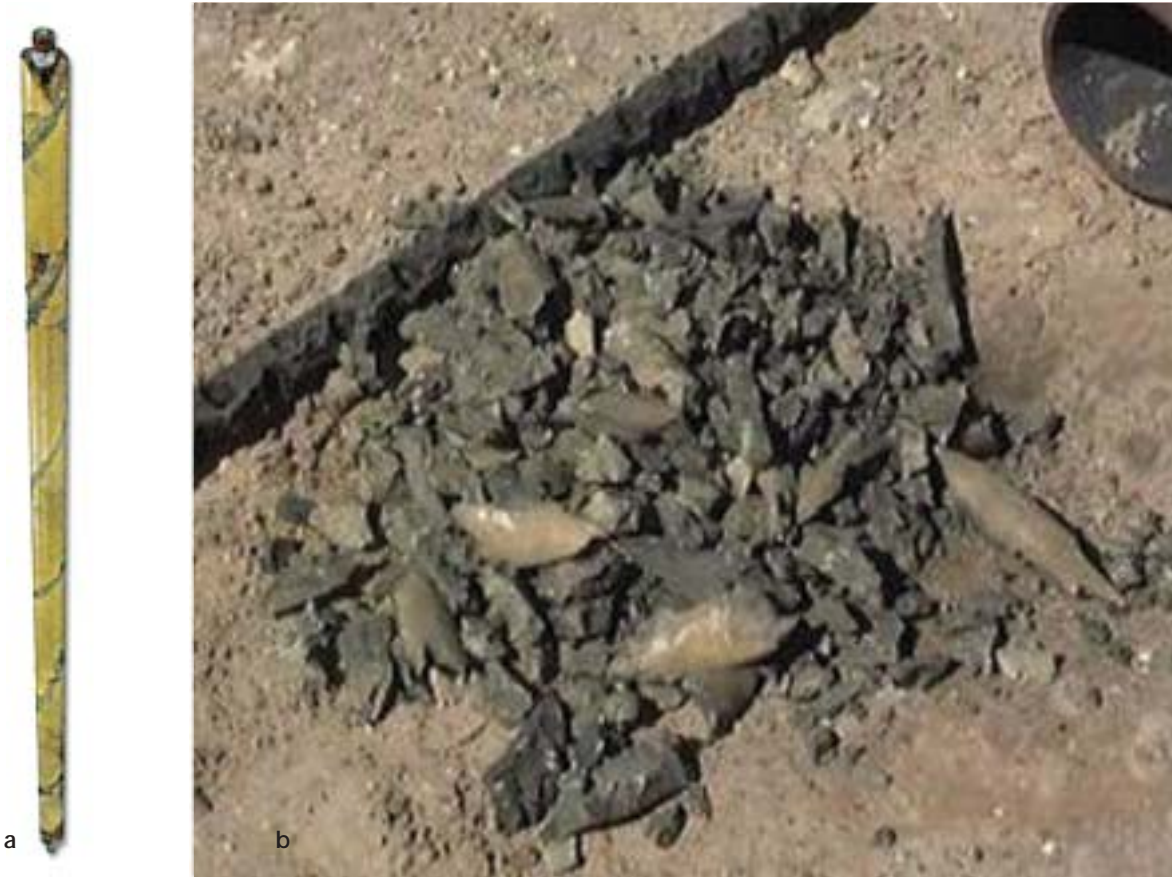
Figure 2 – (a) View of the StimTube™ tool after detonating cord wrapped around the exterior of the tool was ignited – note that essentially none of the tool was ignited by the detonating cord. (b) View of the StimTube™ tool after detonating cord was run through the central ignition tube and ignited. The ignition of the detonating cord resulted in fragmentation of the tool and minor ignition of some of the fragments.
