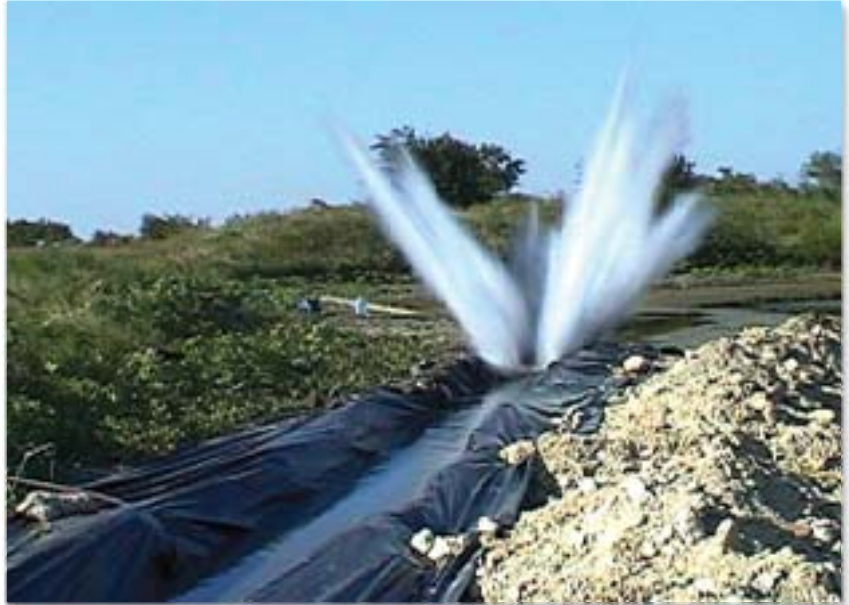
Figure 1 – Surface Test – StimGun™ assembly, 2½ in. (73 mm) Perforating Gun, 6 spf (20 spm), no ignition of StimGun sleeve observed.
